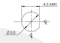
RECOMMENDED TORQUE FOR PANEL NUT: 0.34 - 0.57Nm MAXIMUM PANEL THICKNESS: 3mm
