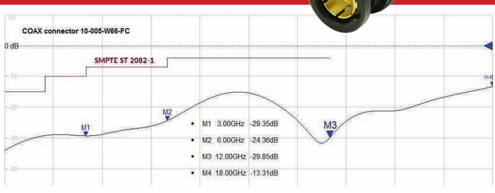
Now successfully tested to provide low loss performance up to 12GHz and in some cases 18GHz. The latest series of BNCs from COAX are perfect for new broadcast applications.
