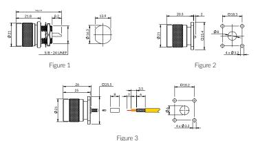
Assembly Procedure - APO19 (25-322-A3), see www.coax-connectors.com/ap for details
