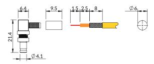
Assembly Procedure - APO17, see www.coax-connectors.com/ap for details
