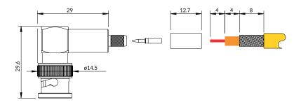
Assembly Procedure - APO19 APO02 (4 Part), see www.coax-connectors.com/ap for details
