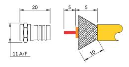
Assembly Procedure - APO09, see www.coax-connectors.com/ap for details
