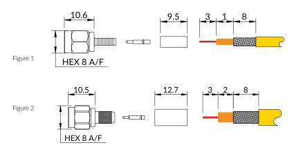
Assembly Procedure - APO01 & APO04 (solder), see www.coax-connectors.com/ap for details
