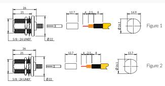
Assembly Procedure - APO01 & APO36 (5 part) APO33 (Direct Solder) See www.coax-connectors.com/ap for details
