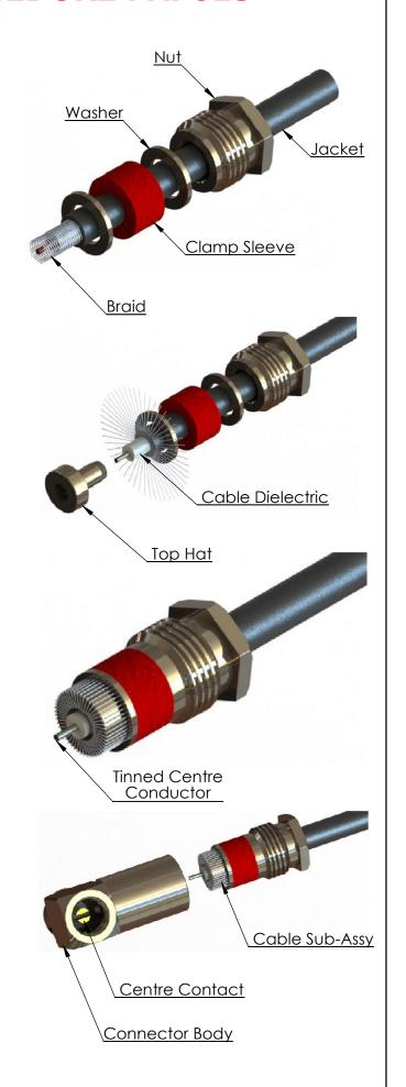
Carefully place Cable sub-assembly into the Connector body, checking that the tinned Centre conductor is correctly place in the slot of the Centre Contact. Carefully slide the Washer and Clamp sleeve forward up to the Top Hat Contact. Then carefully slide the second washer and Nut forward and engage the thread. Using a suitable spanner to hold the Connector body, carefully tighten the Nut to the recommended torque given on the connectors datasheet. Thus clamping the cable in place.
