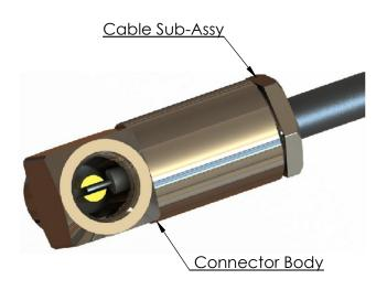
8. Checking the Centre Conductor is still in position in the slot of the tinned centre conductor, carefully heat the Centre Contact using the appropriate tool, so that the solder melts, adding additional as required. Care should be taken not to overheat the contact to avoid damaging the Insulator or cable dielectric. Allow to cool and inspect joint. Screw Cap inplace and tighten.
