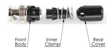
3. Slide the Rear Cover and then Inner Clamp over cable. Position the Inner Clamp so that the end of the Cable Jacket passes through and is level with the end of the Clamp. All of the braid should be visible as shown.
