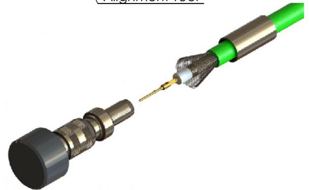
9. Slide the cable into the connector and push home until the centre contact "CLICKS" into place in the connectors dielectric. Ensure all the braid strands pass outside over the knurled area of the connector.
